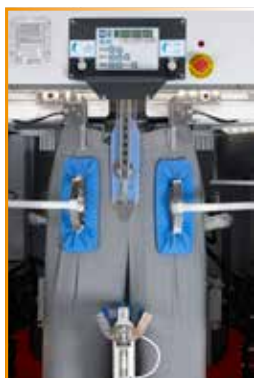
Pleat clamps with pre-steaming function.
